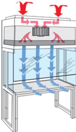
Room air (in red) enters the system from above the HEPA filter; 99.99% particle-free air is forced downward toward the work surface.
