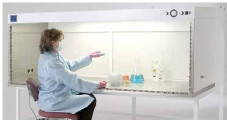
**Horizontal laminar flow hood, with rear-mounted fan/filter unit.**
