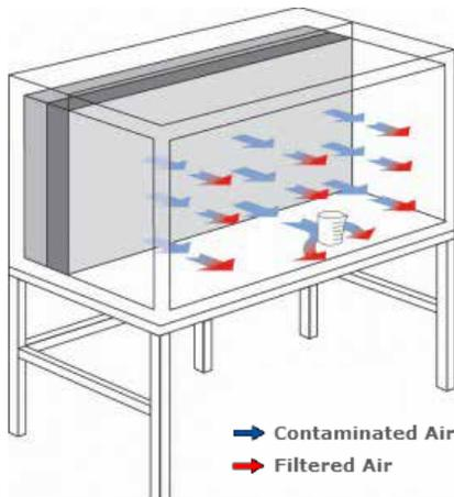
Room air (in red) enters the system from behind the HEPA filter; 99.99% particle-free air is forced in a back-to-front direction across the work surface.
