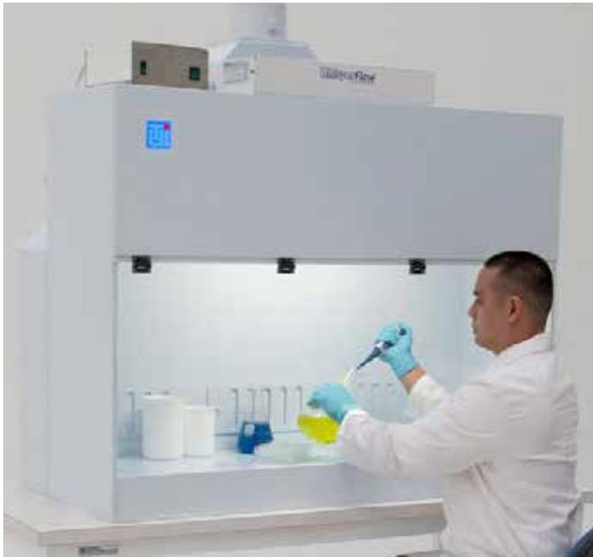
**Vertical laminar flow hood with top-mounted fan/filter unit. Model shown includes rear exhaust baffles and a perforated base to optimize laminar flow, and an overhead duct to feed exhaust air to an in-house ventilation system.**
