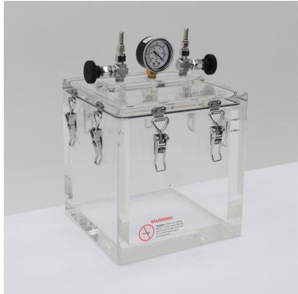
Figure 1. Acrylic vacuum chamber
