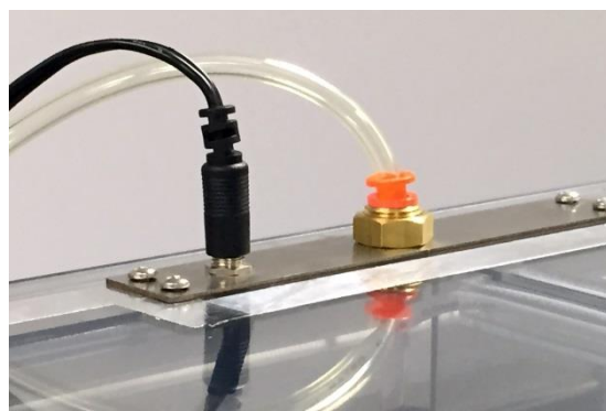
Power supply and nitrogen gas connections
