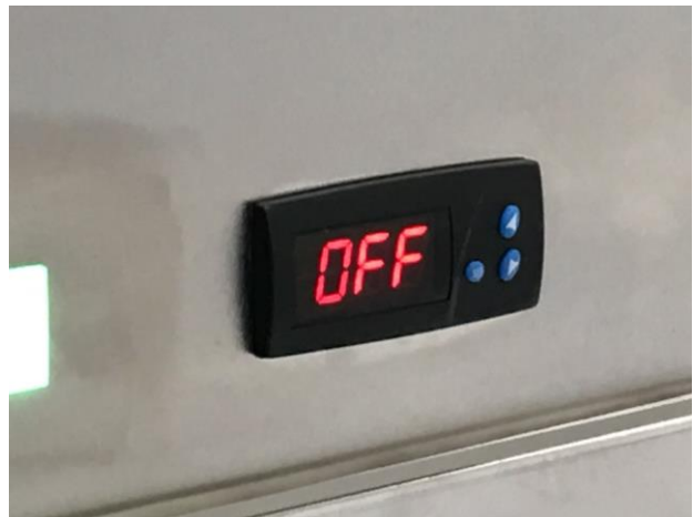
Figure 11: Cycle time can be adjusted via the timer on the "dirty"-side of the pass-through
