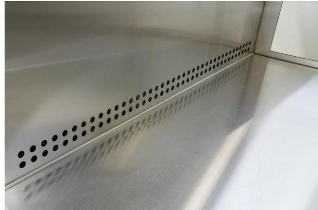
Figure 13: Air escapes through the exhaust vents along the bottom of the chamber
